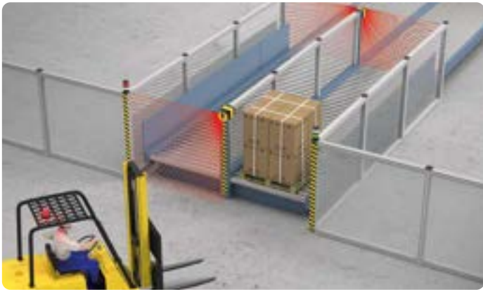
SX5 software configuration allows zone switching for full, right-side and left-side safety protection during this forklift access application.
